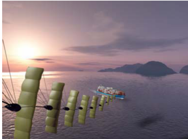
Fig.1 Kite system designed by students from the TU delft to propel a container vessel
