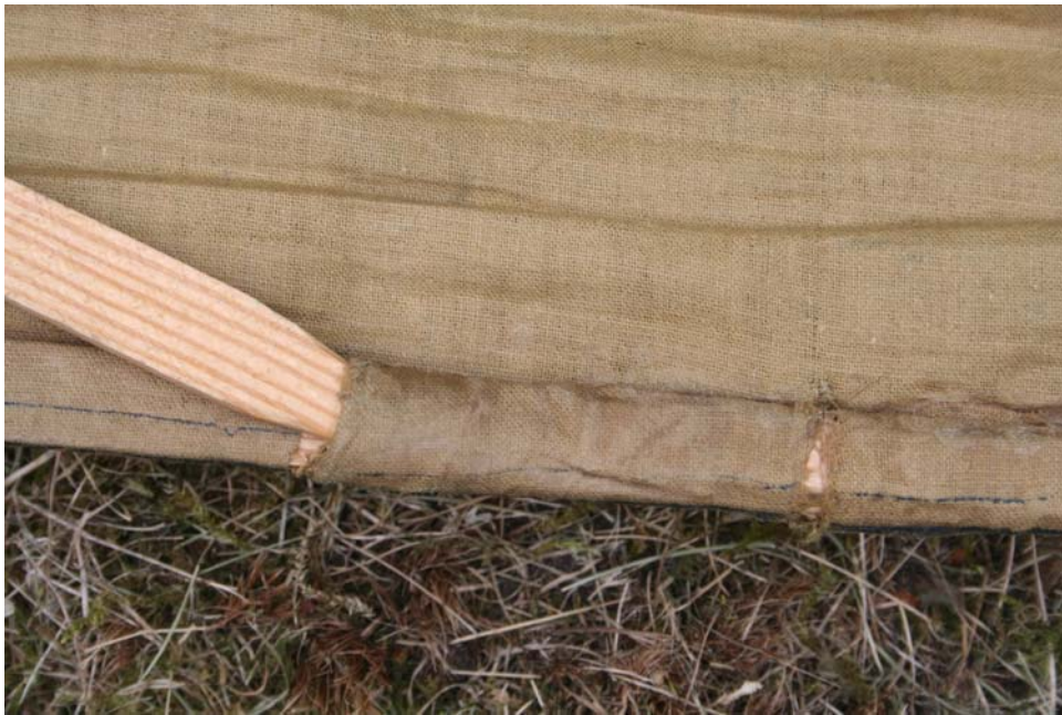
You can see the damage in the cloth caused by the broken stick - the repair itself is hardly visible
