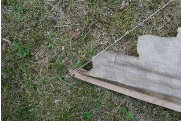
Fixation of the left tension line between tail and lower end of the wing spar
