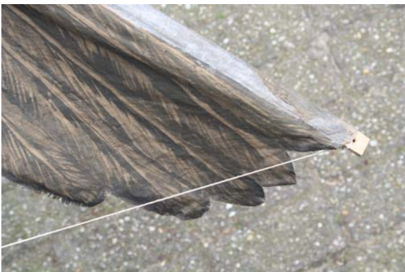
Tension line connected at the tip of the wing spar
