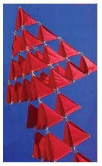
provide reliable stability. He conducted simultaneous tests of different designs, and admitted that the kite with a full complement of cells behaved in the air like "a water logged vessel," while the "hollowed" version acted like "a cork dancing upon the waves."
