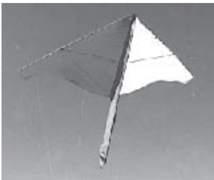
A rigid keeled on-the-wind kite obtains lift from wind striking the lower surface.
