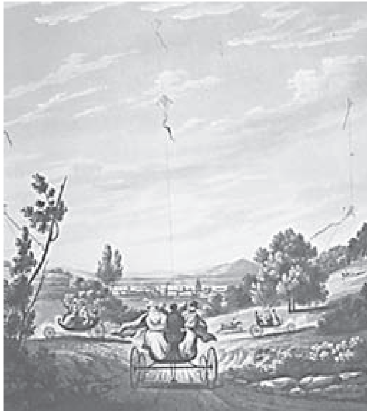
Three Pocock char-volants pulled by kites traveling in various directions, e.g. tacking with the wind.
