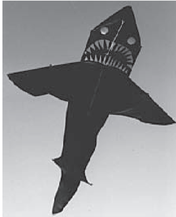
A kite 120 inches deep and 78 inches wide has an aspect ratio of 3.15.
