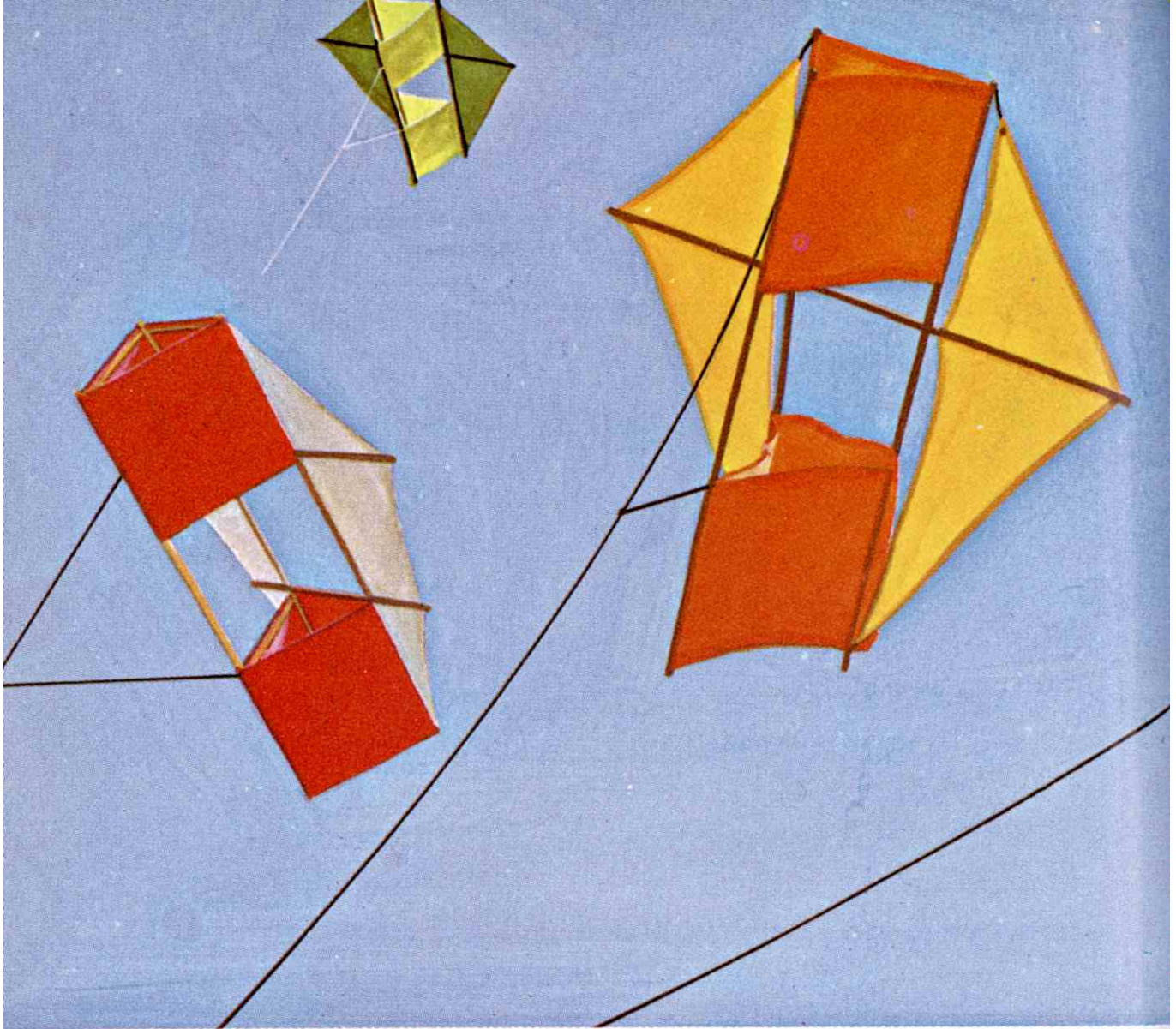
A fleet of French Military (Conyne) Box Kites, all different in number of spars, in rigidity and bracing, and in positioning of spars. Only
