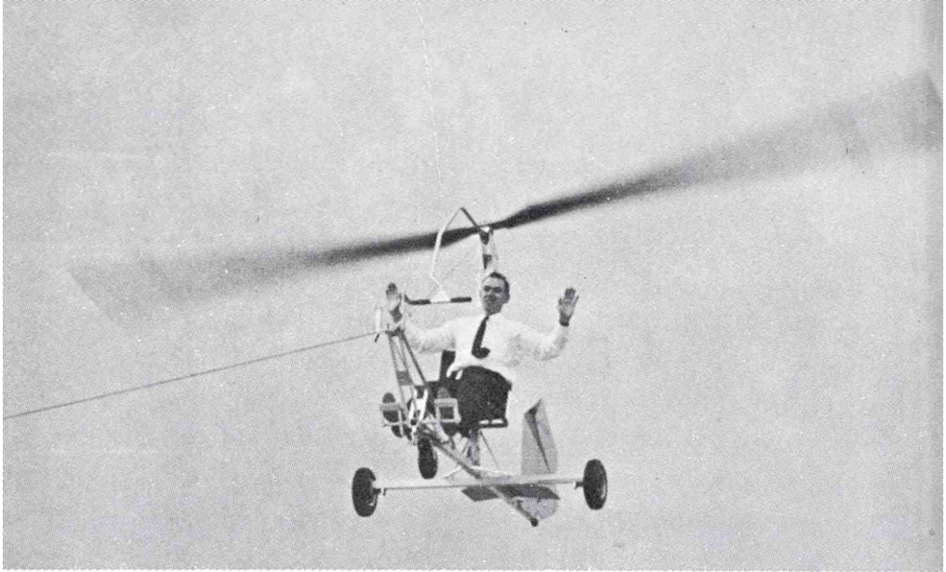
Towed into a light wind, the Bensen Gyroglider becomes a man-carrying kite.
