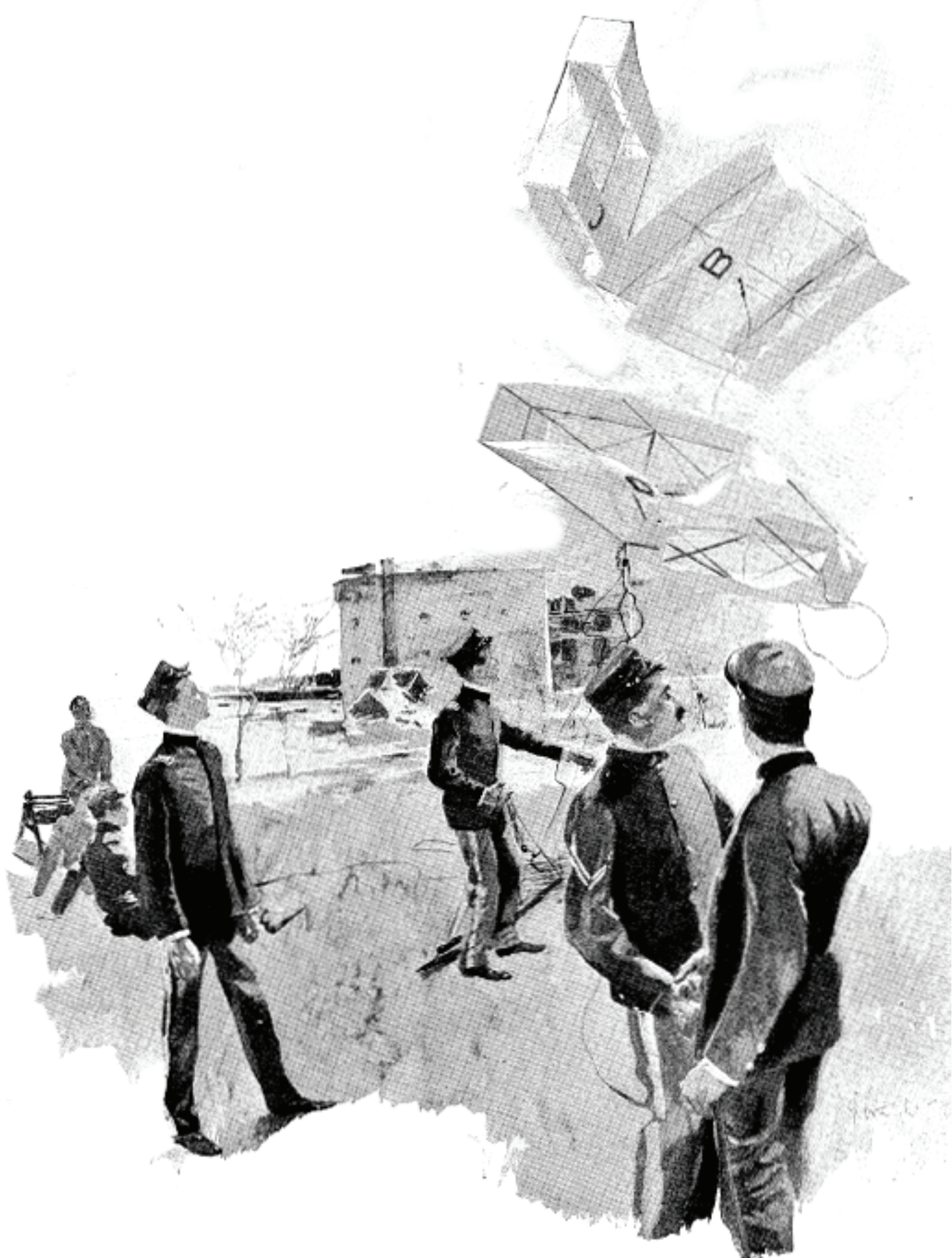
A sketch of one of several incidences faced by Lieut. Wise demonstrating the dangers faced by aeronautical pioneers. As he stepped into the boatswain's chair the lead (pilot) kite collapsed in a sudden gust and the entire kite train came crashing to the ground.
