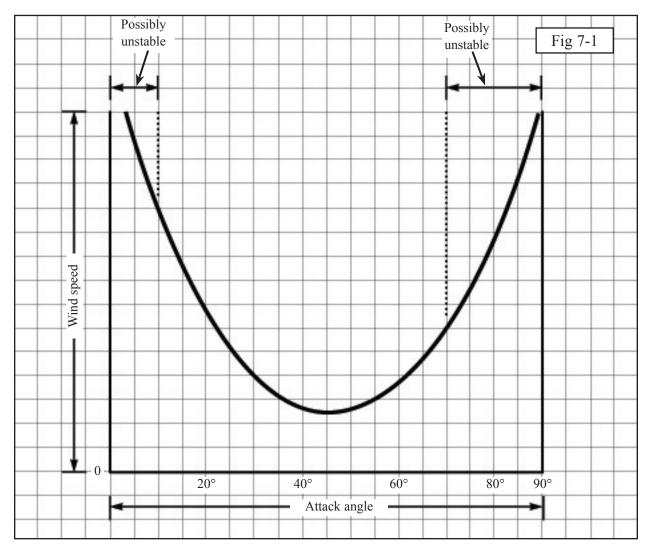
Attack angle vs minimum lift off wind speed and high wind instability (Guesstimated!).
