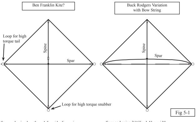
Spar and spine lengths = 1.5 x side dimension Spar 3/16" Diameter, Spine 1.4" Self Bowed to 1/8 of kite diagonal Spar and spine 3/16" x 1.41 x width Bow 1/8 of diagonal. Tow point is stick coupler.
