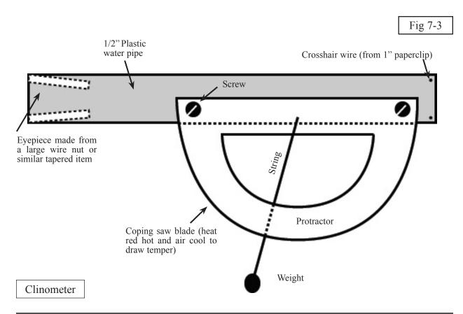
in the air, don't cool it with water or the blade will be re-tempered.
