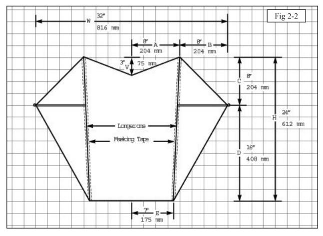
NOTE: If 1/8" ID bar straws are used for longerons, tape them down with 3/4" wide masking tape.
