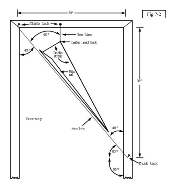
System for accurately setting attack angle of Diamond Kite Two point bridle for 40. The Kite may be held above the reference line as shown here or below. Adjust tow point so the kite sail is parallel to reference line.
