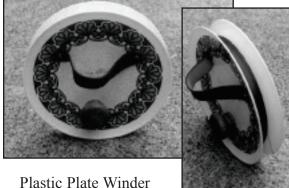
Figures 10-2 and 10-3 show three line holders/winders. One of them is made from two tin-plated steel pie pans that I picked up in a thrift store. After bolting the pans together, I fitted the assembly with a leather wrist strap and a wooden drawer pull knob to hold onto. A second holder/winder was made from two tough plastic dinner plates bolted together and fitted with a leather wrist strap and holding knob.
